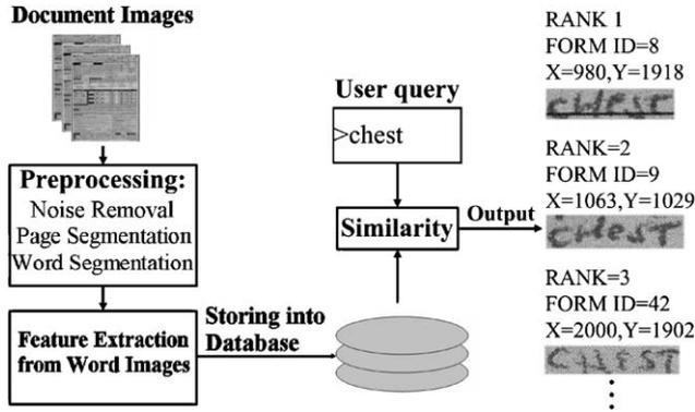
Fig. 1. Diagram of the keyword spotting system.
